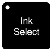
The LED indicator in the key and the Ink Indicator LED corresponding to the first component ink will be illuminated, i.e. PANTONE Yellow. The legend 'ADD' and the amount of ink to add will be shown on the main display.
